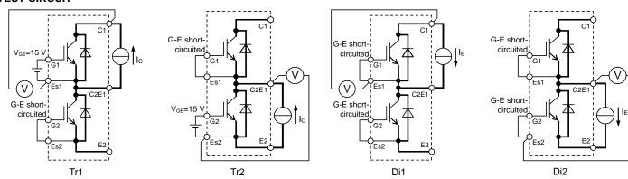
V<sub>CEsat</sub> characteristics test circuit
